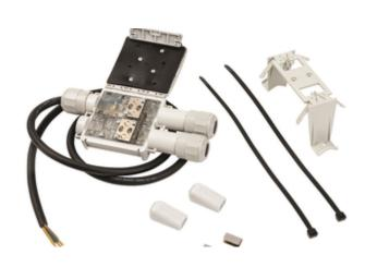
nVent RAYCHEM RayClic connection system is a simple, fast and reliable set of connection kits developed for select nVent RAYCHEM XL-Trace, IceStop and HWAT self-regulating heating cables. No heat guns or wire stripping are needed, because insulation displacement technology is used to make the electrical connection.
