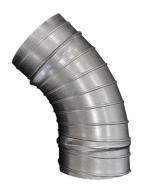
Low pressure and friction loss. Meets SMACNA gauge requirements. Airtight 4-ply lock seam construction. Meets leakage Class 3 for 10" W.G. Duct construction class in a sample test section. Sealant is required only where elbows attach to the duct, saving labor time. Greater structural integrity. 26 ga Galvanized Steel
