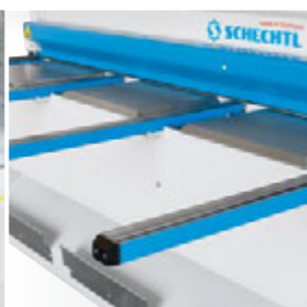
Exchangeable boxes for various cutting materials
